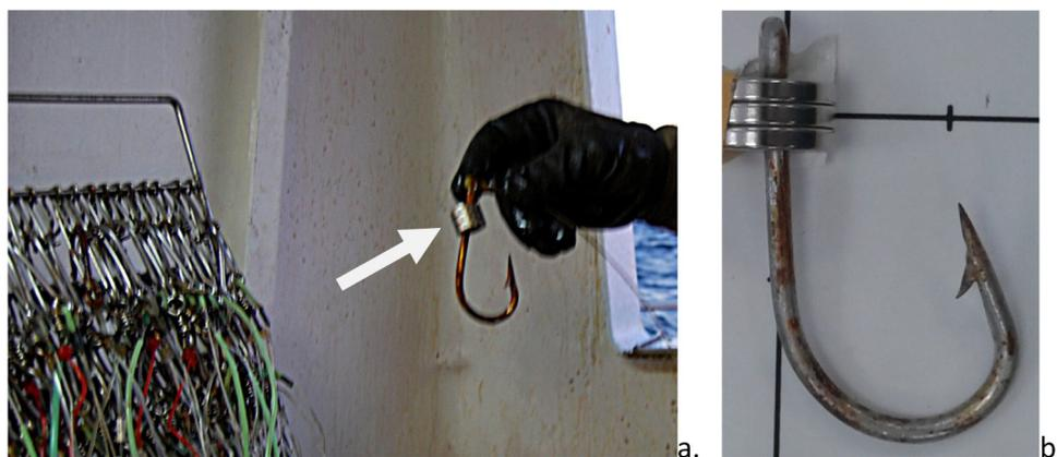
**Fig. 2.** (a) Position of the model 2 magnet with a hook under real fishing conditions. Photo: Sebastián Biton Porsmoguer. (b) Position of model 2 magnet on a hook measured for magnetic field in laboratory. Photo: Christophe Almarcha.
