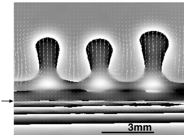
FIG. 4: Superposition of the interferometry figure and velocity map at time 85 s for the fingers of Fig.3. The black arrow denotes the line of initial contact between solutions. The maximum velocity measured by PIV is  $132 \mu\text{m/s}$ .
